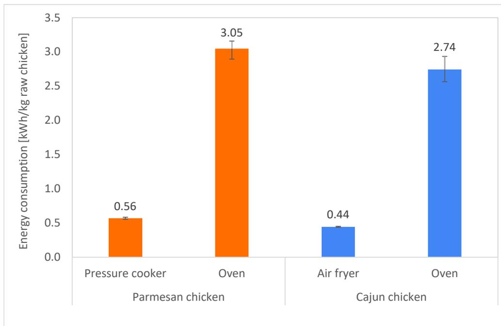
*Figure 1 Comparison of energy consumption between pressure cooker and air fryer against electric oven using two chicken-based recipes; results are presented per kg of raw chicken. Solid bars show mean values, while error bars represent maximum and minimum values from the tests*
