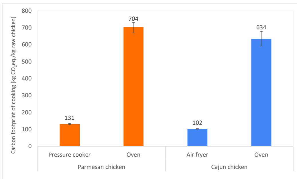
*Figure 2 Comparison of the GHG emission associated with the energy used by a pressure cooker and an air fryer against an electric oven when cooking two chicken-based recipes; results are presented per kg of raw chicken. Solid bars show mean values, while error bars represent maximum and minimum values from the tests.*
